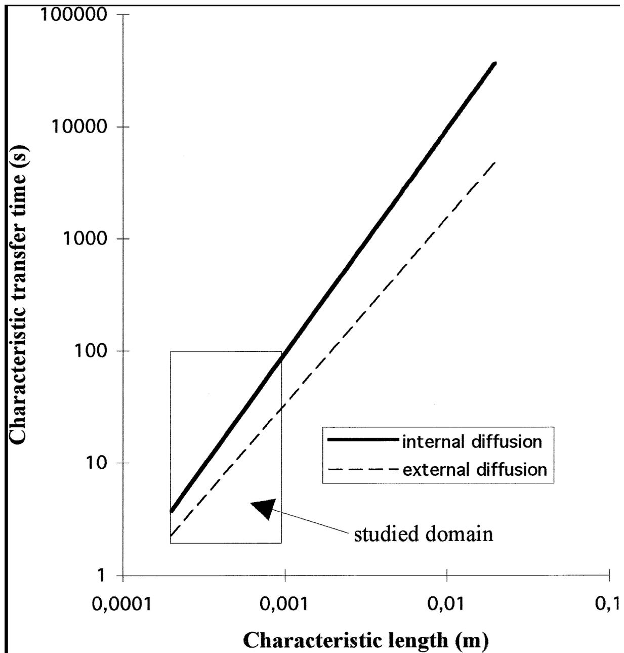
Figure 4 : Influence of the characteristic dimension of aggregates on both external and internal transfer times.
