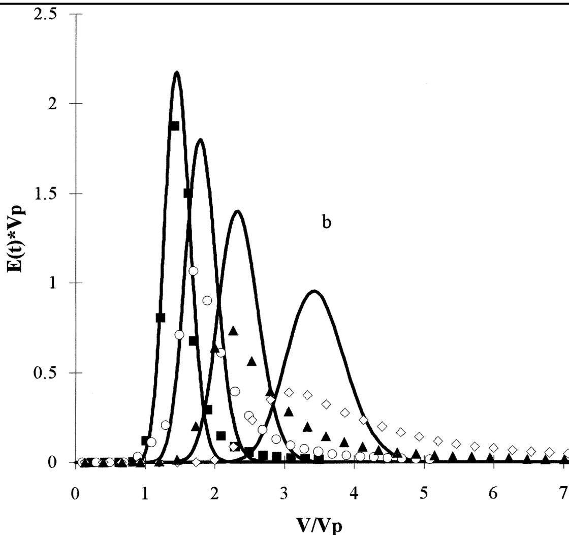
**Figures 1 : breakthrough curves of Np(V) in 1M NaClO<sub>4</sub> with 0.2 M [CO<sub>3</sub>]<sub>t</sub>.**
