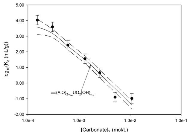
**Fig. 5** Effect of carbonate on U(VI) sorption onto  $\alpha$ -alumina ( $T = 22\text{ }^{\circ}\text{C}$ ;  $[\text{NaCl}] = 0.1\text{ M}$ ;  $\text{pH} = 8.33$ ;  $[\text{Al}_2\text{O}_3] = 1\text{ g L}^{-1}$ ,  $[\text{U(VI)}] = 3.10^{-10}\text{ M}$ ). The fit curves are simply obtained using the sorption data for  $\text{UO}_2\text{Cl}^+$  and  $\text{UO}_2(\text{OH})_{\nu_{\text{OH}}}$  and the data for solution complexes of the ligands.
