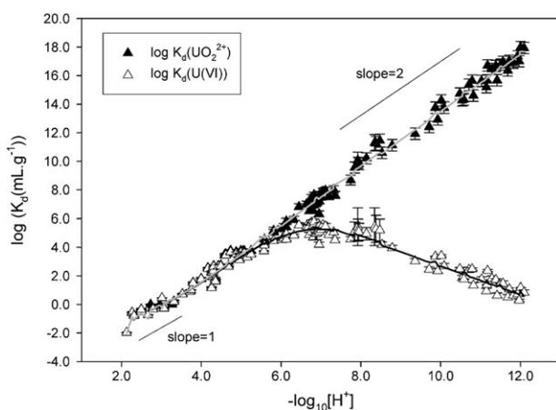
**Fig. 1** Distribution coefficient of U(vi) on  $\alpha$ -Al<sub>2</sub>O<sub>3</sub> ( $T = 22$  °C;  $[NaCl]$  and  $[Cl^-]$  variable;  $[Al_2O_3]$  variable,  $[U(vi)] = 3.10 \cdot 10^{-10}$  M).  $K_{d,UO_2^{2+}}$  (black symbols) was calculated with eqn (2) from  $K_{d,U(VI)}$  (white symbols) experimental values and calculated Ringböm coefficient  $\alpha_{UO_2^{2+}}$ . The solid lines were calculated using fitted parameters from Table 2.
