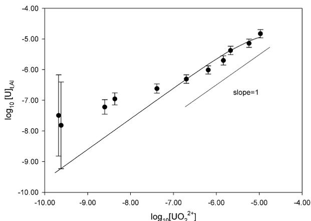
**Fig. 2** Adsorbed uranium(vi) on  $\alpha$ - $\text{Al}_2\text{O}_3$  ( $T = 22^\circ\text{C}$ ;  $[\text{Al}_2\text{O}_3] = 12.5 \text{ g L}^{-1}$ ;  $\text{pH} = 5.0 \pm 0.2$ ;  $[\text{NaCl}] = 0.1 \text{ M}$ ;  $[\text{U(vi)}] = 3.10^{-10} \text{ M}$ ) as a function of  $[\text{UO}_2^{2+}]$ . The solid lines were calculated using the same parameters from Table 2.
