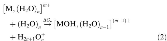
where  $\text{M}^{m+}$  corresponds to  $\text{Be}^{2+}$  or  $\text{BeOH}^+$ .  $\Delta G_n$  corresponds to the Helmholtz free energy cost of the reaction. In the case of  $n \rightarrow \infty$ , Eq. (2) can be written as follows
